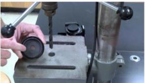
b) hole drilled in an extra body cap
