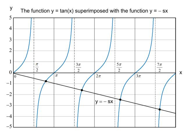
Figure 3. Solving the transcendental equation  $\tan x = -sx$  by superimposing the graphs  $y = \tan x$  and y = -sx. The intersection points are the solutions for the values of x, from which the resonance frequencies are found:  $f = \frac{x}{\pi} f_o$ .
