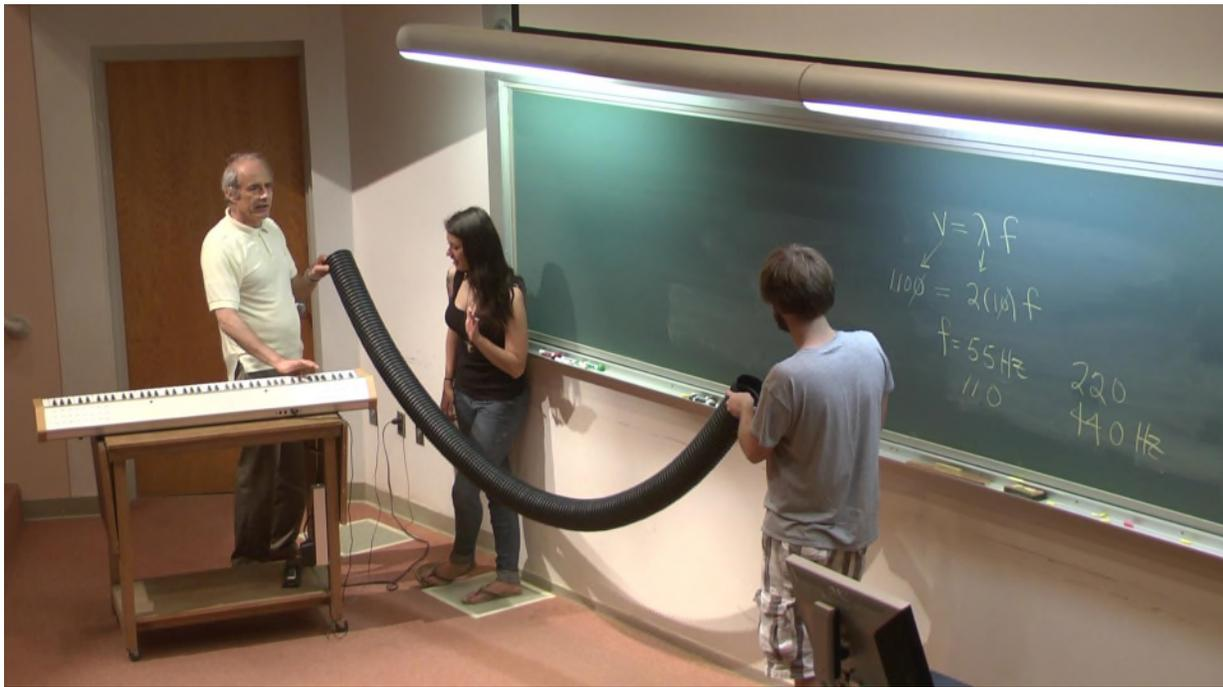
**Figure 1.** The 10 ft (3 m) drainage tube in class. The keyboard is used to match the frequency when the tube is smacked. The matched tone is found to be a semitone lower than the theoretical predicted value of  $A_1 = 55$  Hz.
