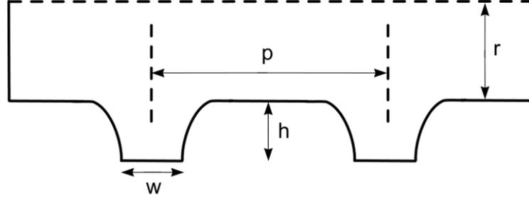
**Figure 5.** Corrugated-pipe section (not to scale) adapted from Nakiboğlu, Belfroid, Golliard and Hirschberg [11] with parameters relevant to the formula giving the speed of sound in the tube.
