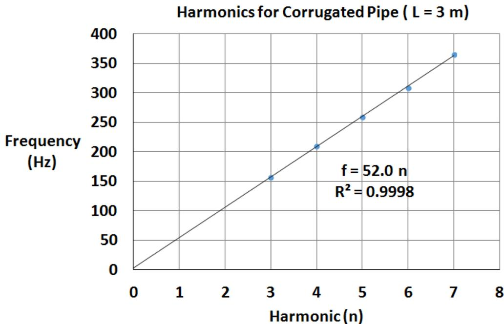
**Figure 6.** Plot of harmonics from twirling a corrugated 3 m (10 ft) pipe over one's head. The linear fit gives a fundamental frequency of 52.0 Hz. The pitches are measured by the free audio software program *Audacity* [10].
