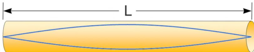
**Figure 2.** Fundamental standing wave in an open pipe. One half-wave,  $\frac{\lambda}{2}$ , fits in the pipe of length  $L$  so that the wavelength  $\lambda = 2L$ , i.e. twice the length of the pipe.
