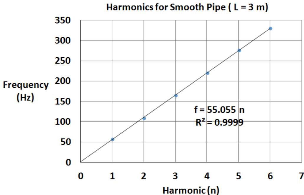
**Figure 4.** Plot of harmonics present in the spectrum when a smooth 3 m (10 ft) pipe is dropped. The linear fit gives a fundamental frequency of  $55.055 = 55.1 \text{ Hz}$ . The pitches are measured by the free audio software program *Audacity* [10].
