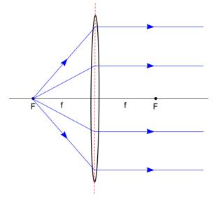
For a thin lens you have one focal length and it is the same on both sides. Light starting out at a focal point F results in parallel light.
