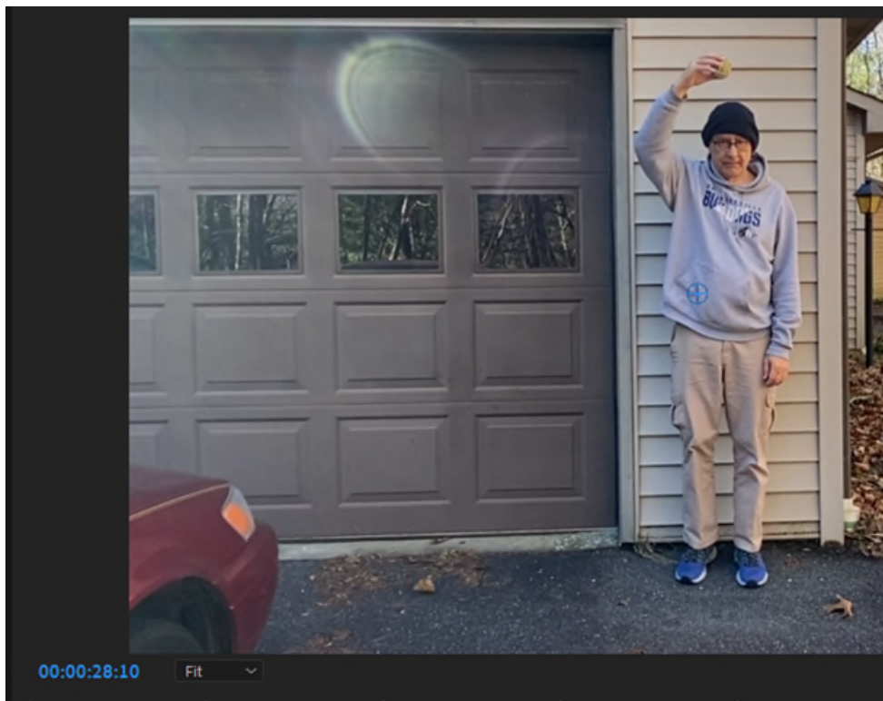
Frame 10 past the 28-second mark on the video with the ball at h = 77 inches = 1.96 meters.
